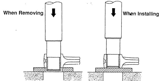
REPLACING THE SMALL END BUSHING
