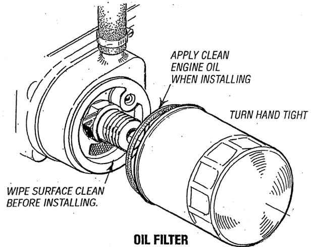
3. **Filling the Oil Sump.** Add new oil through the oil filler cap on the top of the engine or through the side oil fill. After refilling, run the generator for a few moments while checking the oil pressure. Make sure there is no leakage around the new oil filter or from the oil drain system, and stop the engine. Then check the quantity of oil with the lube oil dipstick. Fill to, but not over the high mark on the dipstick, should the engine require additional oil.
