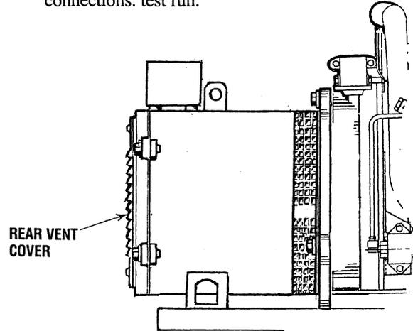
2. With the aid of a sling or fabricated lifting eye, support the stator housing assembly and carefully guide it over the rotor assembly until the rear bearing contacts the bearing boss in the rear support.
