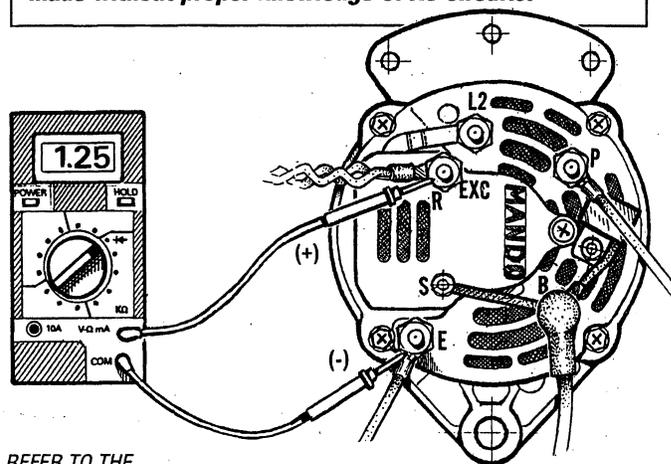
REFER TO THE WIRING DIAGRAMS FOR THE ABOVE WIRING HARNESS CONNECTIONS
