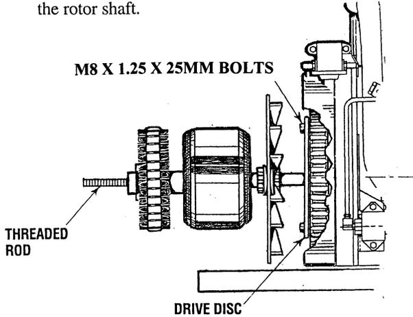
4. Rotate the generator by hand two full revolutions to ensure the generator rotates freely. Reinstall the rear vent cover.
