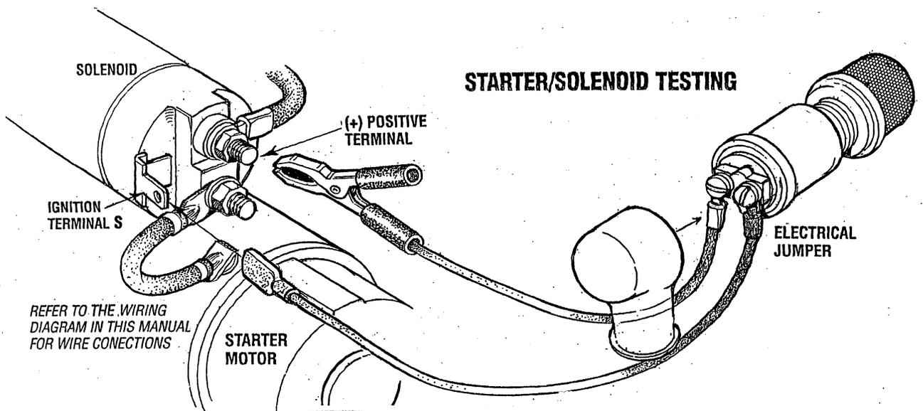
REFER TO THE WIRING DIAGRAM IN THIS MANUAL FOR WIRE CONNECTIONS
