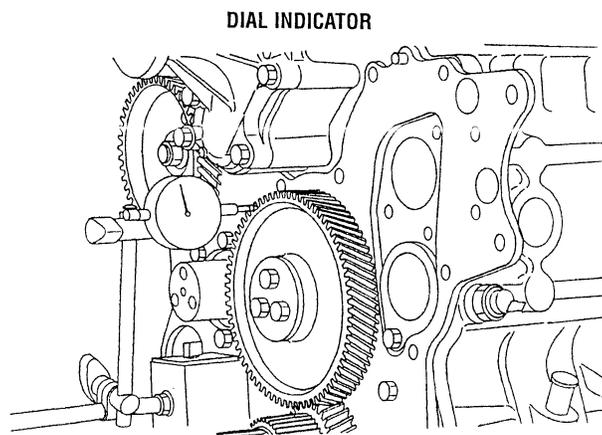
MEASURING GEAR SIDE CLEARANCE
