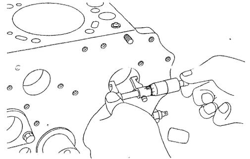
MEASURING THE CYLINDER BORE I.D.
