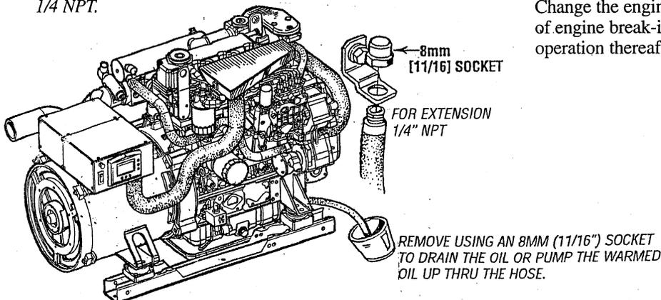
2. **Replacement of the Oil Filter.** When removing the used oil filter, you may find it helpful and cleaner to punch a hole in the upper and lower portion of the old filter to drain the oil from it into a container before removing it. This helps to lessen spillage. A small style automotive filter wrench should be helpful in removing the old oil filter.
