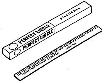
Application : Use to check the oil clearance between crankshaft and bearing, etc..
