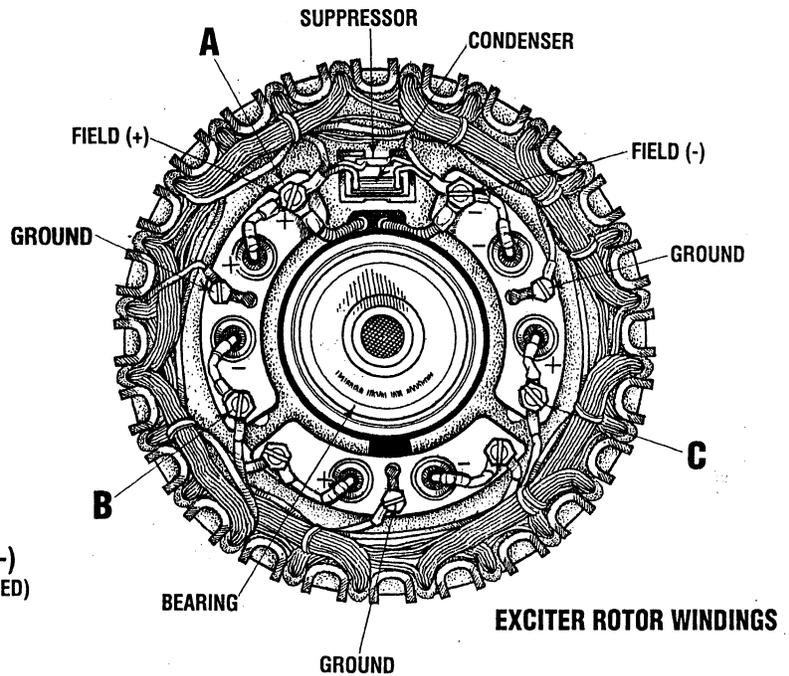
Disconnect these three wires from the diode bridge plates taking care not to drop any screws or washers.
